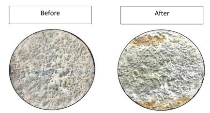
The very nature of Krystaline technology to enhance the hydration of C-S-H crystals and gels even years after the concrete has been placed makes it the perfect product to self-heal cracks in the presence of water.
